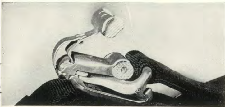
Step Two. When contact with the ground or water is made, the buttons should be squeezed and clip rotated out and down.
