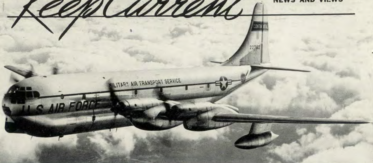
Faster and more economical. One of these YC-97J Stratofreighters, powered by T-34 turboprop engines, flew the Atlantic in six hours.
