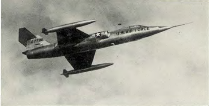
The F-104 is the only jet fighter using a downward ejection seat.
