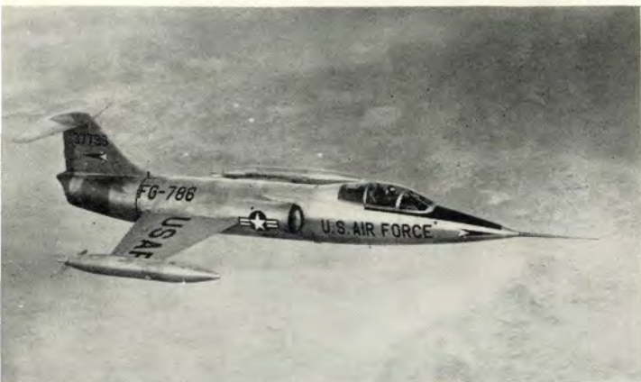
The T-shaped horizontal stabilizer has no elevator and moves as a unit.
